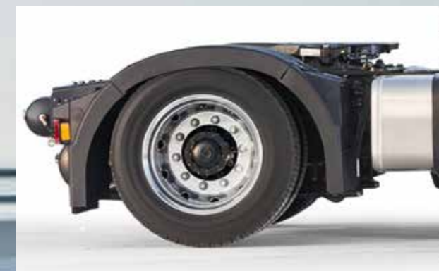
Low Liner: You can also choose the Low Liner version with a 5 th wheel height that can be lowered down to 940 mm as preferred.
