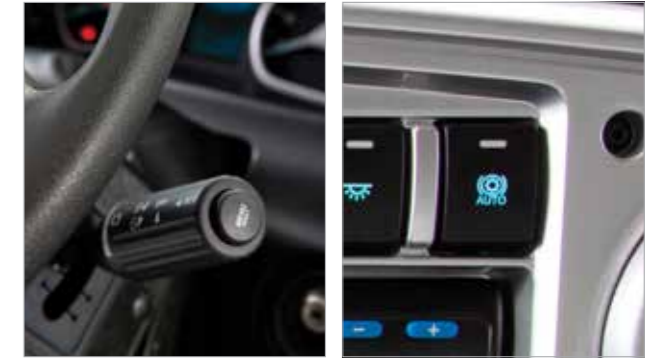
Engine brake and Intarder operating lever: You can manually activate the auxiliary brakes, or you can enable the vehicle to set it automatically for you.
